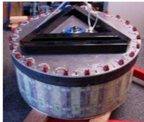
Figure 11. (a) Manufacture of single coils (b) Single coils mounted inside steel ring (c) Completed stator winding.
