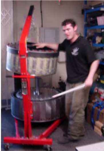
Figure 12. Final assembly of the stator winding into the C-core rotor.
