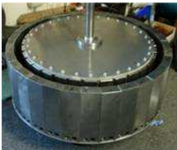
Figure 10. (a) C-core with magnets mounted (b) Un-machined sections of the C-core (c) C-core sections with PMs mounted (d) Complete C-core rotor.
