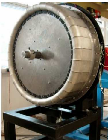
Figure 7: 15kW C-GEN prototype on test at Edinburgh University
