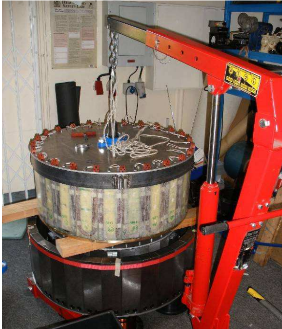
Figure 6: Lowering the 'C' core stator to meet the rotor is simpler and safer than for a conventional PM machine.
